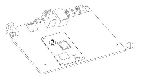
b) Insert the four black nylon washers from the side of the gap between the four corners of the CM4 Module and the PCB. The mounting holes of the four nylon washers should be aligned with the four mounting holes of the CM4 Module. The nylon washer has two sizes, 1.5mm height\*6mm diameter and 3mm height\*6mm diameter, which are to support 1.5mm or 3mm height 100pin board to board connector correspondingly.
