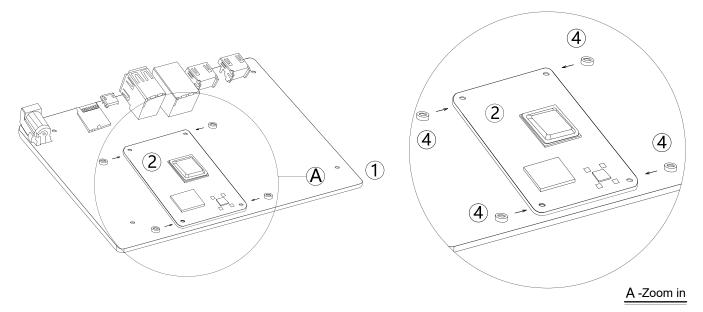
c) . When the three thermal conductive silicon pads on the CM4 Cooler are aligned with the three components on the CM4 Module, attach CM4 Cooler with CM4 Module. Fix them on the CM4 IO board by screwing screws from the bottom of base board.
